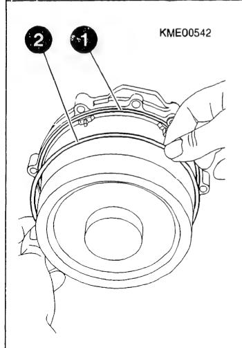
ASSEMBLING ALTERNATOR Alternator leak test Parts required \* 6 × hexagon bolt M6×35 DIN 933-8.8: comm. avail. \* 12 × washer DIN 125-A 6.4: comm. avail. \* 6 × hexagon nut M6 DIN 934-8: comm. avail. \* 1 × B+ connecting cable nut: vehicle-specific
